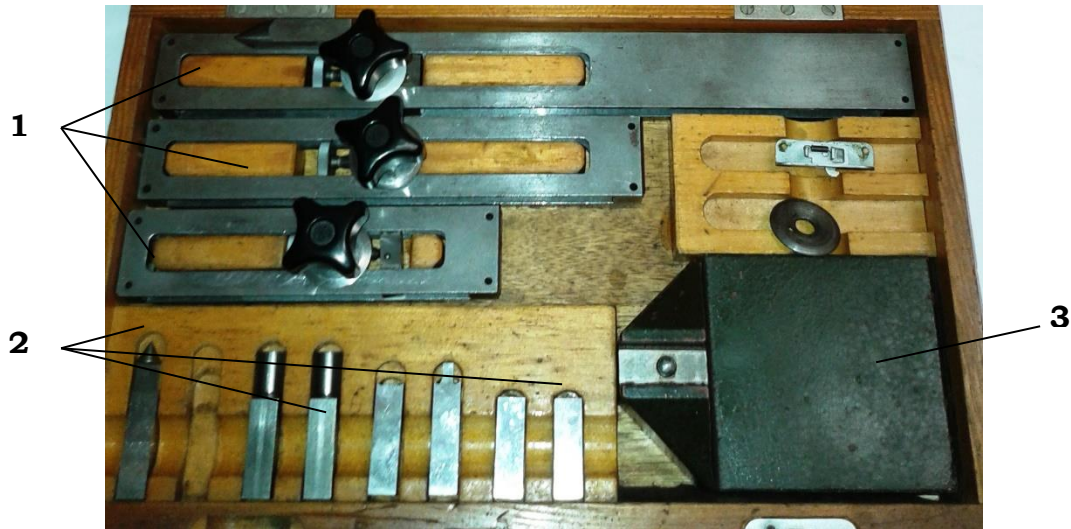
Fig. 3. Gauge block accessories set
