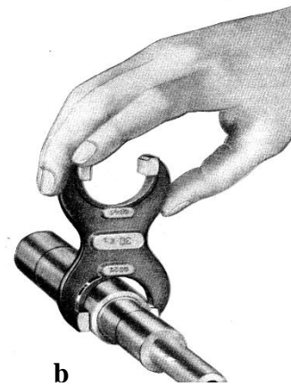
Fig. 7. Checking with double-jaw snap double-ended gauge
